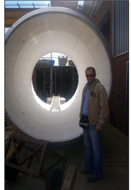
Ceramic fibre blanket rated up to 1420°C
