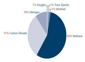
produced during the decomposition of waste is a potent contributor to the global green house affect and also pose significant health and safety risks. Thus must be treated and due to it's often rich in methane content represent a potential energy source which can be used to produce energy.
