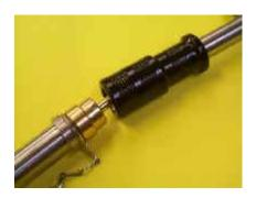
3. Plug the Sample Cylinder into the Bayonet Adaptor on the Pump. The Filling Indicator (if being used) is fitted between the Pump and the Sample Cylinder.
