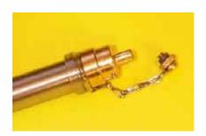
2. Check Sample Cylinder is empty by depressing Schrader Valve in the Cylinder Head against the Pump Handle Retaining Bolt Head.
