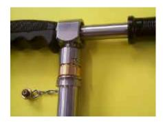
4. The Cylinder should now be purged by pumping up to pressure several times and releasing the contents of the cylinder as in 2 above. With Double Ended Cylinders the Purging Attachment can be used. The Attachment is fitted to the "free" end of the cylinder and the pump "pumped" several times to enable sample to flow through to atmosphere. The Attachment is removed before the sample is taken.
